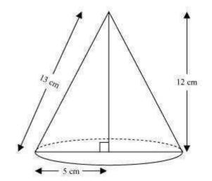
When right-angled  $\triangle$ ABC is revolved about its side 12 cm, a cone with height (h) as 12 cm, radius (r) as 5 cm, and slant height (l) 13 cm will be formed.
