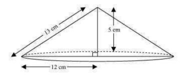
When right-angled  $\triangle$ ABC is revolved about its side 5 cm, a cone will be formed having radius (r) as 12 cm, height (h) as 5 cm, and slant height (l) as 13 cm.
